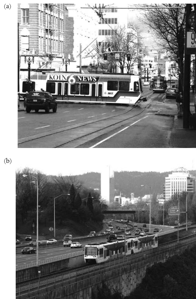
Figure 2.17. Photo (a) shows a “light” rail Portland MAX vehicle operating like a streetcar in the foreground with a true light rail streetcar in the background. Photo (b) shows Portland’s MAX line outside of the central city, where it travels large distances more typical of a light rail system. (Credit: available under the Creative Commons Attribution 2.5 License)
